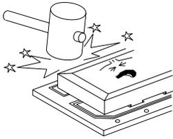
LCD may be shifted or conductive rubber may be reshaped, which will cause defects.
